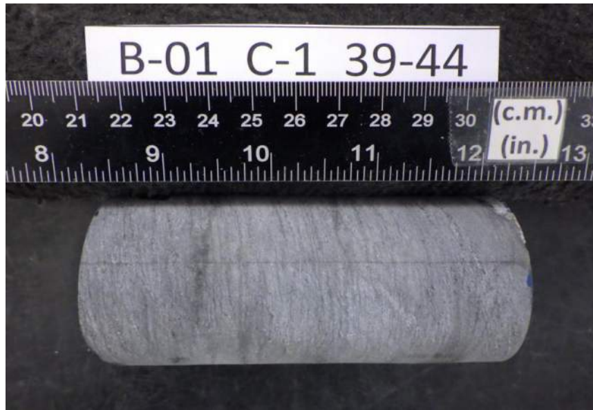
After cutting and grinding
